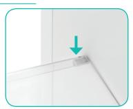
**b.** Latch Middle Shelf onto the sides of the metal bolts.
