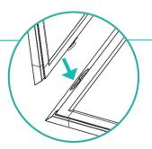
**c.** Insert circular pegs from side panel into circular slot.
