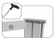
**e.** Connect the top extrusions together and use torx key to tighten.
