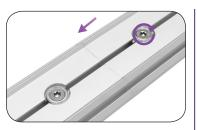
**a.** Split Connector: Slide into side of 60D extrusion channel that faces the frame's middle. Then attach other extrusion onto the Split Connector. Tighten screws with included torx key.
