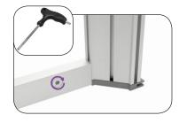
**e.** Connect bottom extrusions together and use torx key to tighten.
